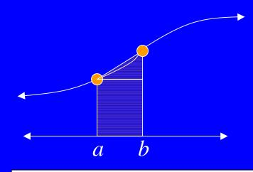
Interpolation function derived at endpoints of interval by a straight line (polynomial of degree one)
