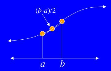
Interpolation function derived at endpoints and midpoint of interval by a quadratic (polynomial of degree two)
