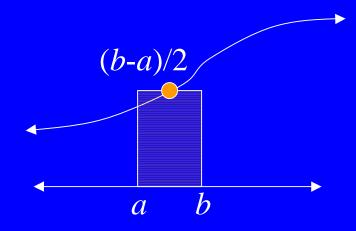
Interpolation function derived at midpoint of interval by a constant (polynomial of degree zero)
